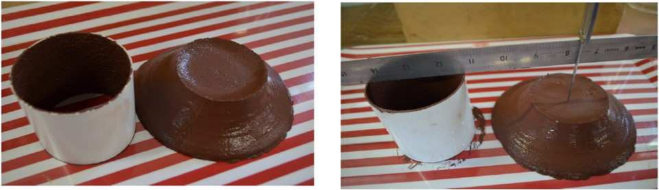
FIGURE 7: BOGER SLUMP TEST
