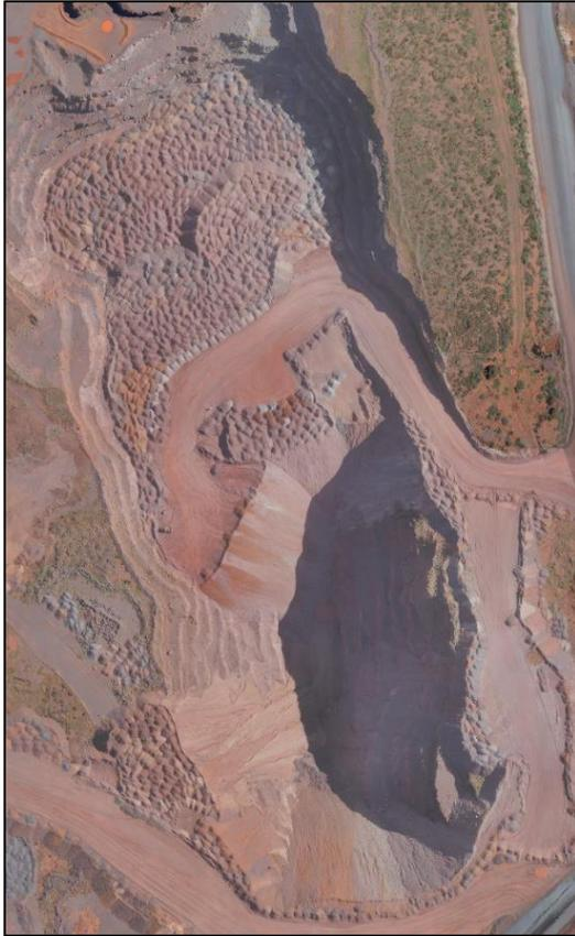
Pit KM02 was depleted in April 2020, after which it was utilised as Compartment 3b of the Paste Disposal Facility.
