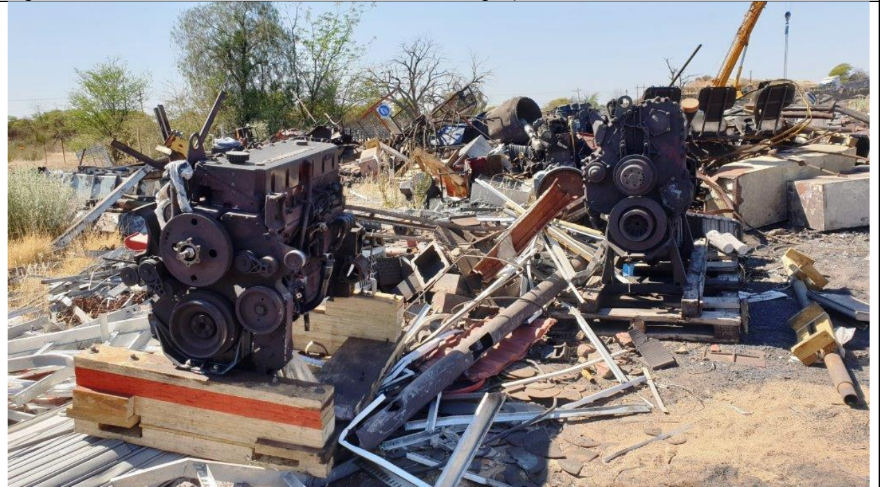
Figure 6.9: Scrapped Engines at Black Rock salvage yard not stored in bunds
