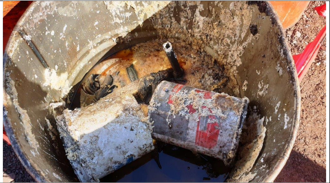
Figure 6.16: Nchwaning 3 Emulsion waste stored outside of bunded area.
