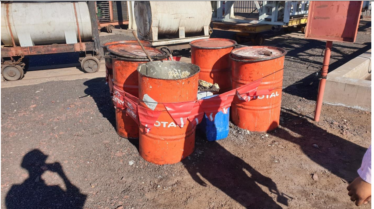
Figure 6.15: Nchwaning 3 Emulsion waste stored outside of bunded area.
