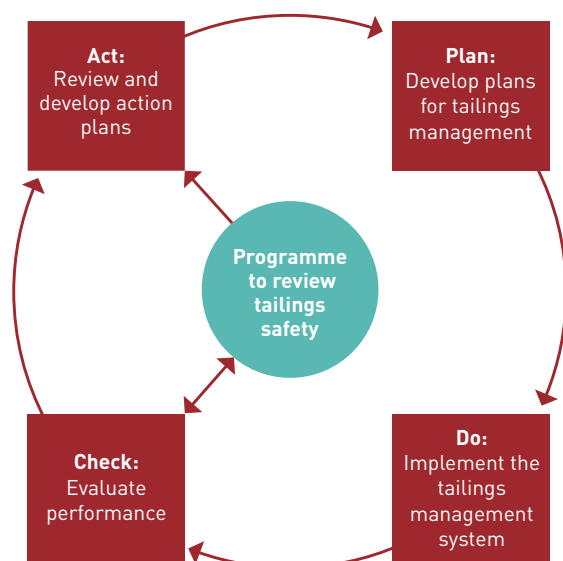
Figure 5: Integration of a programme for tailings safety review into the tailings management system
