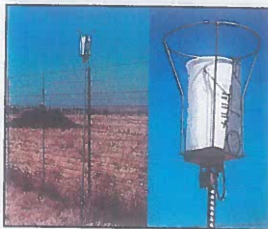
Figure 2-37: Single dust bucket monitors as established for BKM Mine
